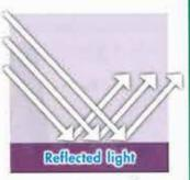
An object with a rough surface reflects light differently than an object with a smooth
