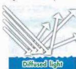
surface. When light strikes a rough surface, the light rays bounce off at the same angle but in many different directions. The reflected light is diffused. Diffuse means to go in all
